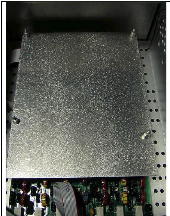
Figure 8 - Installation of four 1/4" spacers on top of shield
