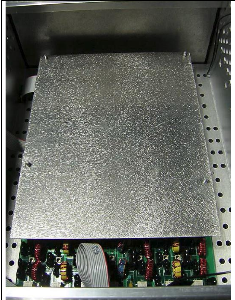
Figure 6 - Placement of RF shield on top of 1" spacers
