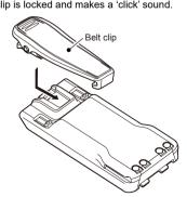
Lift the tab up (1), and slide the belt clip in the direction
