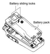
1. Push both battery sliding locks in the direction of the arrow. (1) The battery pack is then released.
